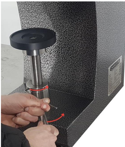
Left: Loosening coupling nut
